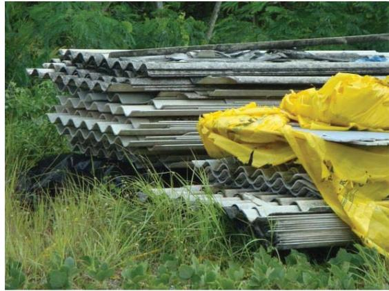
*Examples of asbestos used in construction in the Pacific Islands*
